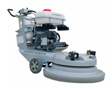
Lavina B36-GTS is a powerful machine designed for concrete grinding and polishing, same as deep cleaning on the big projects.
