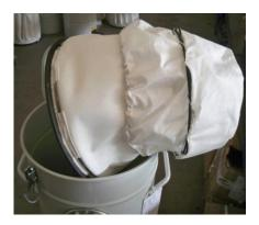
➤ Loosen the clamp and remove the polyester dust filter. The same procedure should be used to remove the polypropylene filter for vacuuming liquids. Fit the new filter and tighten with the clamp. Fit the entire assembly in the container. Fit the float and motor head and secure with the two safety retainers.
