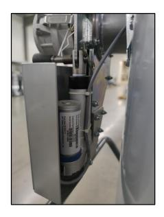
When you are ready and all the components are connected, mount back the top cover and connect the accumulator. Test if the automatic filter cleaning works properly.
