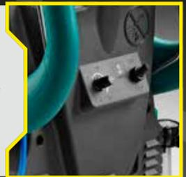
Waterflow adjusting knob and dosing system pump connection.
